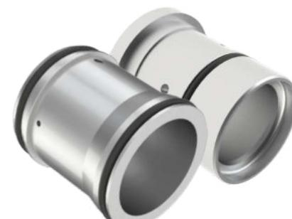
With quenching, atmosphere side with rubber bellow single seals, independent of direction of rotation or as single seal dependent of direction of rotation (right hand)
