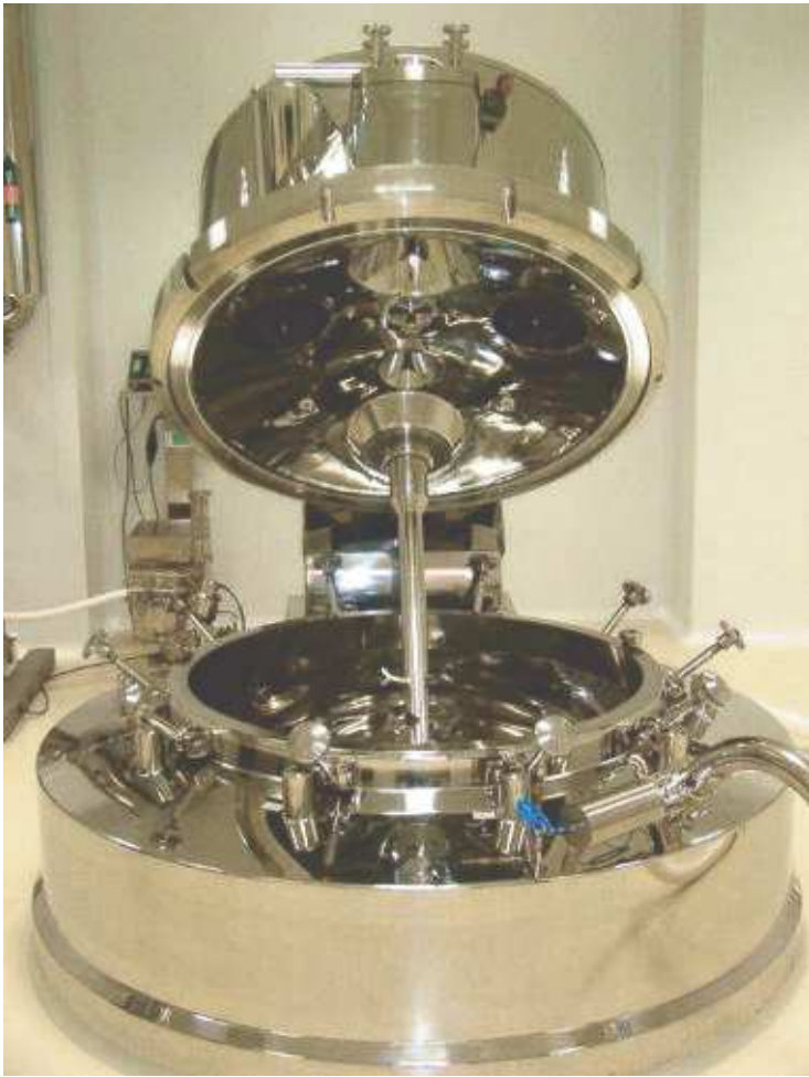
Housing mechanical seal for food, chemical and pharmaceutical processes (Granulierer-Mixer- Dryer from Bio-Inox Pharma®)
